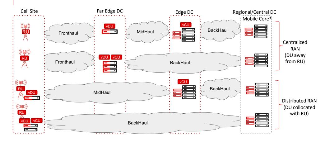
\*Some Mobile Core components (such as UPF) can be moved closer to the subscriber and placed a the Edge DC collocated with the CU as part of Control Plane User Plane Separation (CUPS)
