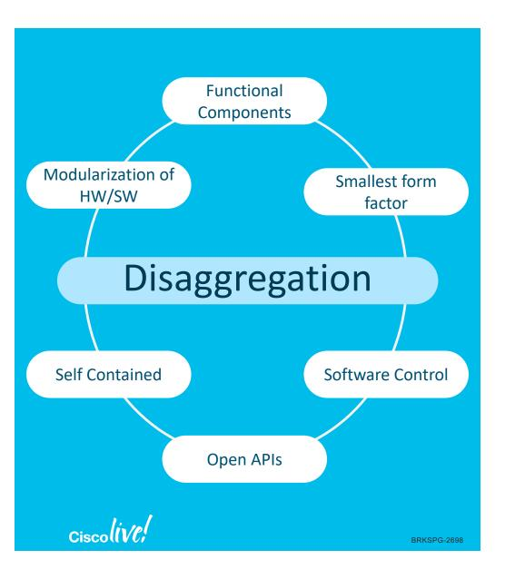
"The separation of networking equipment into functional components and allowing each component to be individually deployed. Ideally, provided in the smallest form factor capable of delivering a specific function. Equipment should be self-contained, required no additional common equipment to operate, and incorporate open APIs to enable Software control
